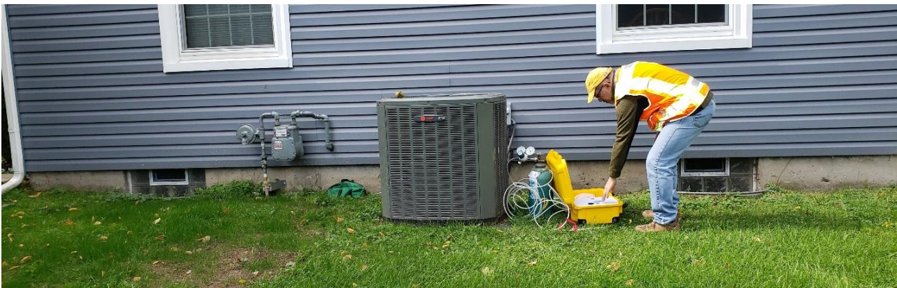
Joe setting up one of the simulated gas leaks
